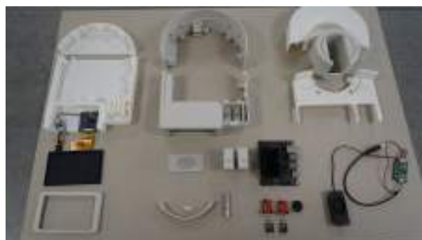
Figure 4.9: All printed components and key circuit modules
