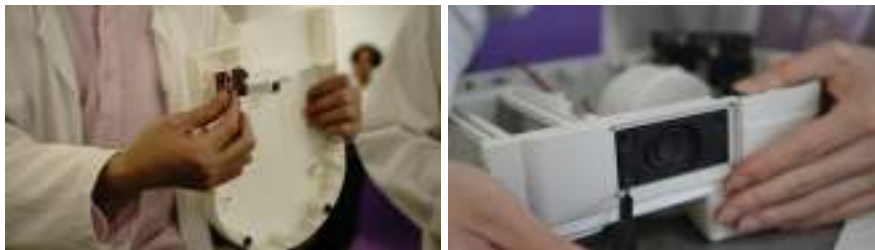
Figure 4.3: Left: Internal support ribs and microswitch slot; Right: speaker cutout;
